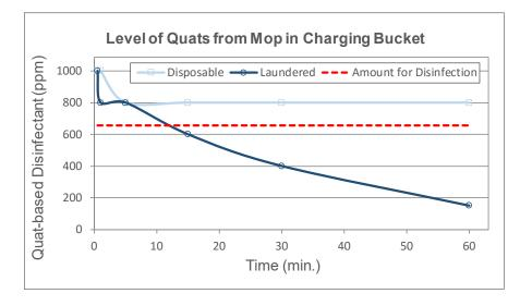
Figure 8 Levels of quat disinfectant in residual solution sampled from the mop when applied using a laundered versus disposable microfiber mop. The delicate structures of microfiber can be damaged by elevated temperatures, bleach-based chemicals and abrasion through mechanical action during the washing and drying process.
